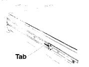
**3.** Press the tab DOWN on the RIGHT side and lift the tab UP on the LEFT side at the same time. Then pull drawer out another inch.
